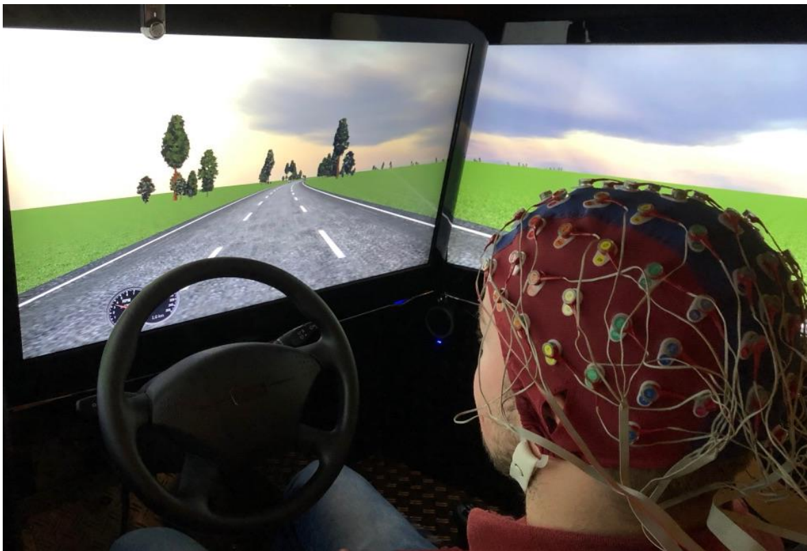
Figure 1. Driving simulator setup with participant wearing 64 electrode EEG cap.
